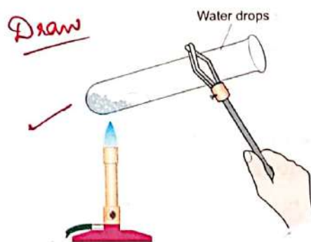
Fig. 8.6 The blue vitriol crystals turn into a white powdery anhydrous salt on being heated.
